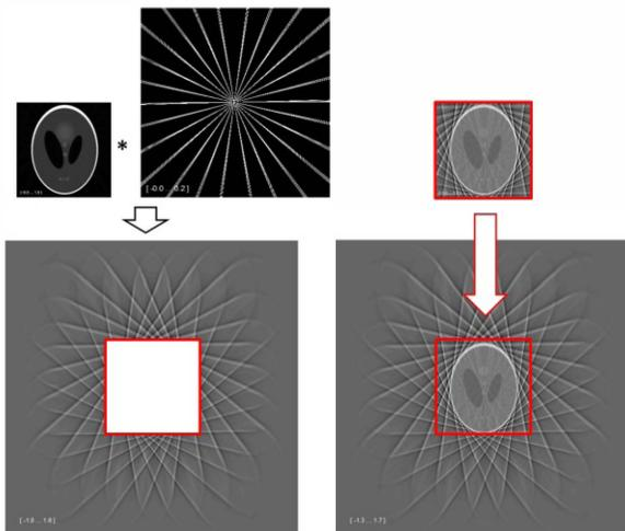
Fig 2. Merging. The ungated reconstruction (top left corner) is convolved with the PSF to obtain a first volume. The central area of this volume is cropped and replaced by the gated reconstruction (top right corner) to obtain a merged volume (bottom right corner).
