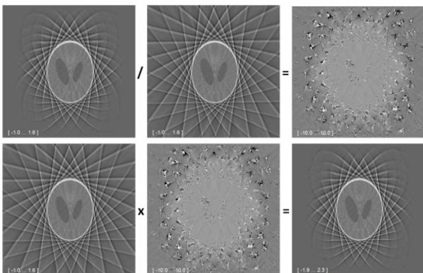
Fig 3. Masking. Volume1 (top left corner) is the convolution of the ungated volume and a small PSF (as large as the ungated). Volume2 (top row, middle) is the convolution of the ungated volume and a large PSF (three times as large as the ungated), cropped to keep only the central area. Multiplying the gated reconstruction with the mask, we obtain a zero-padded-convolution-like volume.
