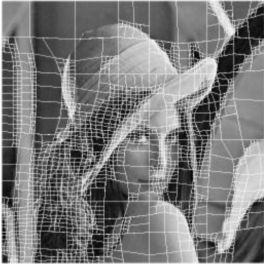
a) Example of mesh generated with an Active Quadtree Mesh Algorithm
