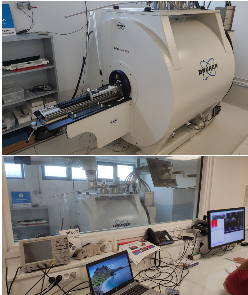
Figure 10: 11.7T Bruker biospec 117/16 USR preclinical MRI machine, part of the PILoT imaging platform and its control room
