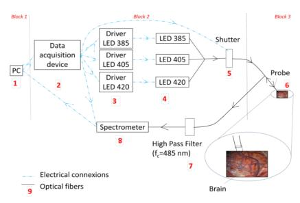
Figure 2: drawing of the new device
