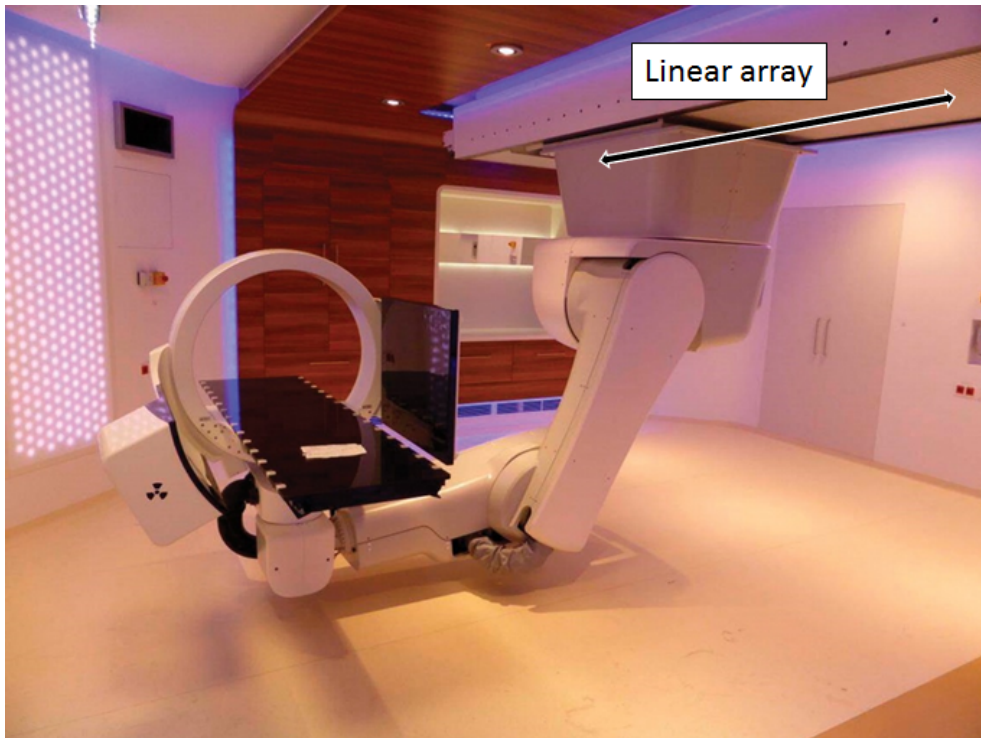
Figure 3.2: picture of the ceiling-mounted robot used at MedAustron . An independently movable X-ray source and a flat panel detector (imaging ring) are mounted directly on the couch. The imaging ring system allows patient imaging before the irradiation for imaging registration purposes. The linear array which allows for translation movements is emphasized.
