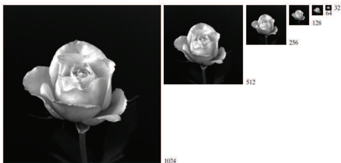
Figure 2.3: Effects of reducing spatial resolution. A 1024x1024, 8-bit image down-sampled to size 32x32 pixels [Gonzalez and Woods (2002)].
