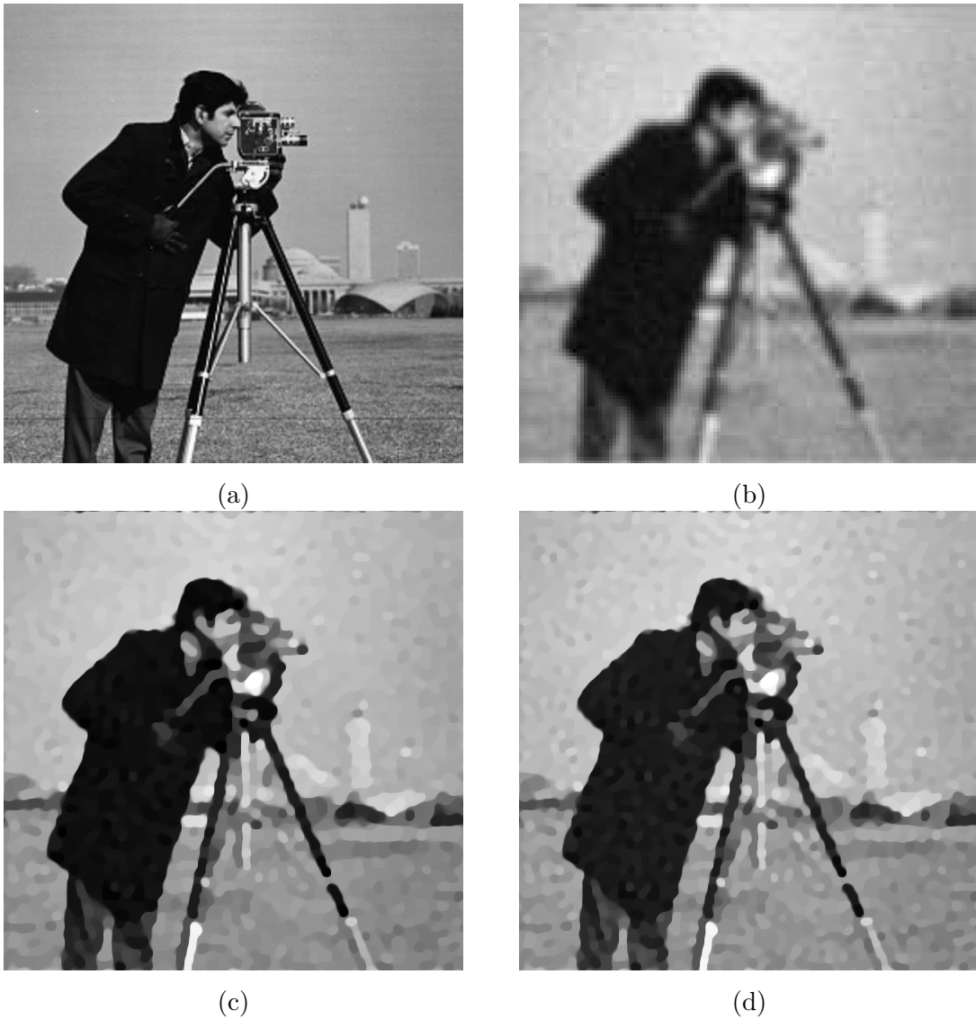
Figure 4.6: (a). Ground truth - Cameraman image; (b). Low resolution blurred and noisy image ( p = 4, \sigma_{blur} = 4.85, \sigma = 4.3 ); (c). Restored image with \mu_{DM} ; (d). Restored image with \mu_{UPRE} .
