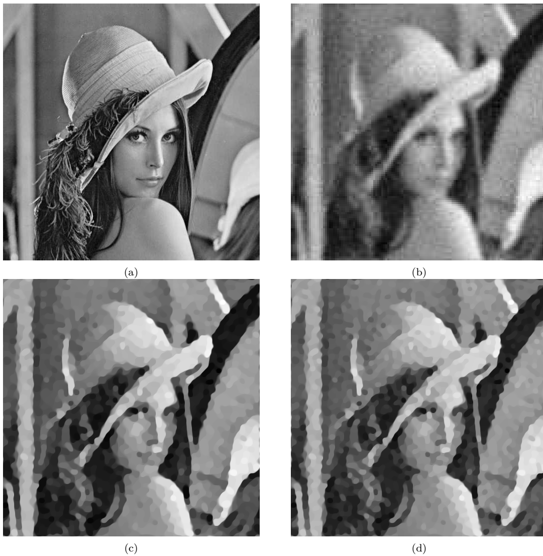
Figure 4.9: (a). Ground truth - Lena image; (b). Low resolution blurred and noisy image ( p = 4, \sigma_{blur} = 4.85, \sigma = 6 ); (c). Restored image with \mu_{DM} ; (d). Restored image with \mu_{UPRE} .
