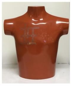
**Figure 3.14.** Anthropomorphic thorax phantom. The phantom is about 50 cm in height with a width and thickness of 28 cm and 19 cm, respectively, at the level of the heart.
