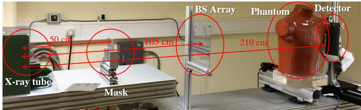
**Figure 6.12.** Prototype x-ray system used for the experiments. The considered air gap between the object and the detector was about 8 cm. The object is depicted in the lateral acquisition position.
