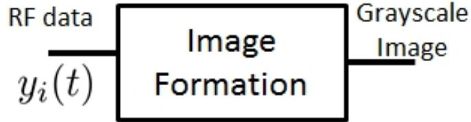
Figure 2.10: The ultrasound image formation block and its corresponding inputs and outputs. The RF data represents all the  $N_{el}$  recorded signals  $y_i(t)$
