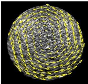
**Figure 2.** Example of estimated motion fields on the rotating disk, speed = 9.8 cm/s
