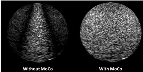
**Figure 1.** B-Mode images of a rotating disk obtained without MoCo (left) and with MoCo (right); Outer speed = 9.8 cm/s
