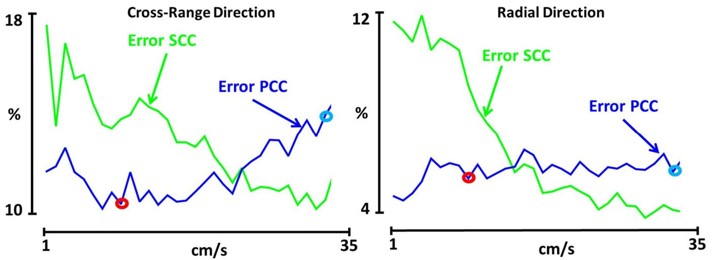
Figure 3. Average normalized errors of the cross-range (left) and radial (right) displacements measured by SCC (green) and PCC (blue). The abscissa represents the outer speed of the disk. The dots refer to the examples illustrated in Figure 4.
