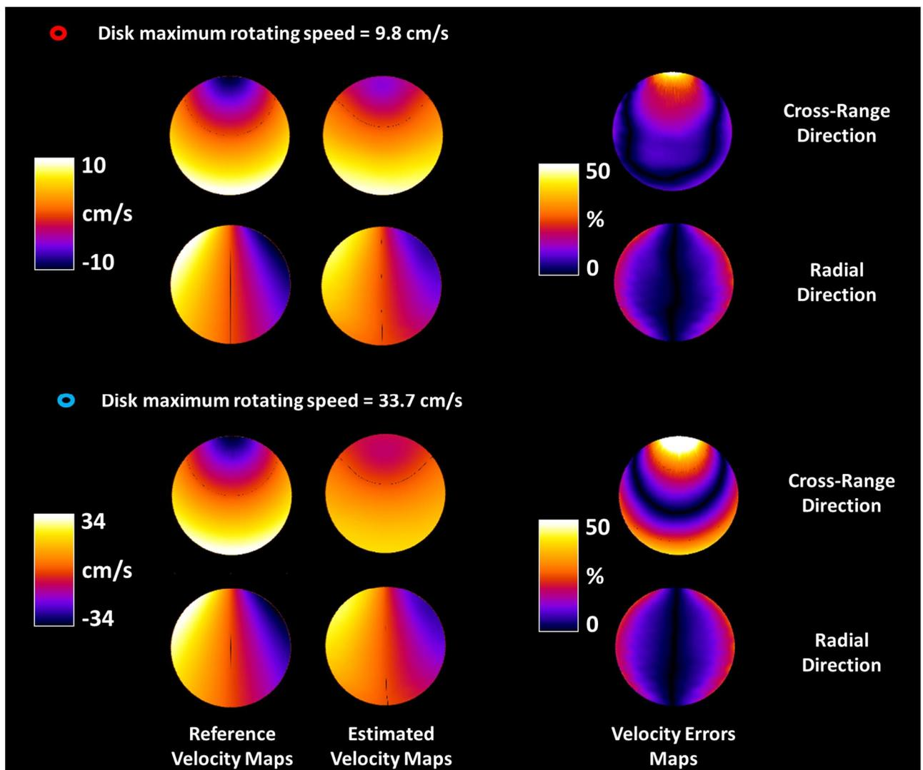
Figure 4. Velocity and errors maps: PCC-derived velocities vs. ground-truth.
