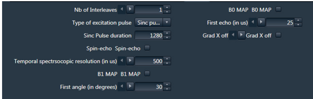
Figure 4.7.: Illustration of the 'Special Card' which is the window interface where the user can manage and modify parameters such as the number of spatial interleaves, the maximum gradients slew rate, whether we want to use an under-sampling or not...
