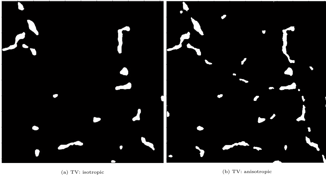
Figure 4.6: Binary sparse bone reconstructed images with 20 projection angles and 729 X-rays per projection with \sigma_p = 6 . (a) isotropic TV: MR_m = 2.35\% ; (b) anisotropic TV: MR_m = 1.41\% .
