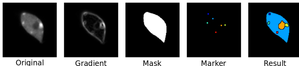
Fig. 5.5 Example of marker-controlled watershed segmentation on an image of a nucleus of Arabidopsis thaliana (image courtesy of Kaori Sakai and Javier Arpon, INRA-Versailles).
