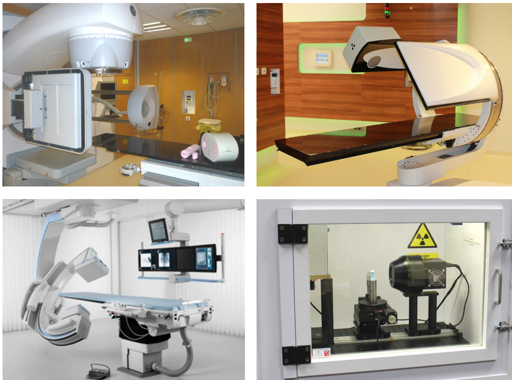
Figure 1.1: Cone-beam CT scanners with a circular source trajectory and a flat panel detector which I have used in my research: Elekta XVI used in [T1, 4, S6] (top left), medPhoton ImagingRing used in [S3] (top right), Philips C-arm used in [S5] (bottom left) and Photonic Science table top system used in [J31] (bottom right).
