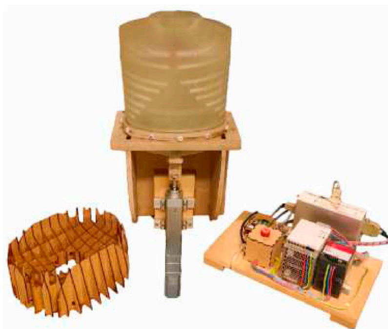
Figure 2. Photograph of the 4D thorax phantom. From left to right: support grid, actual thorax phantom with its hydraulic cylinder and electronic control board.
