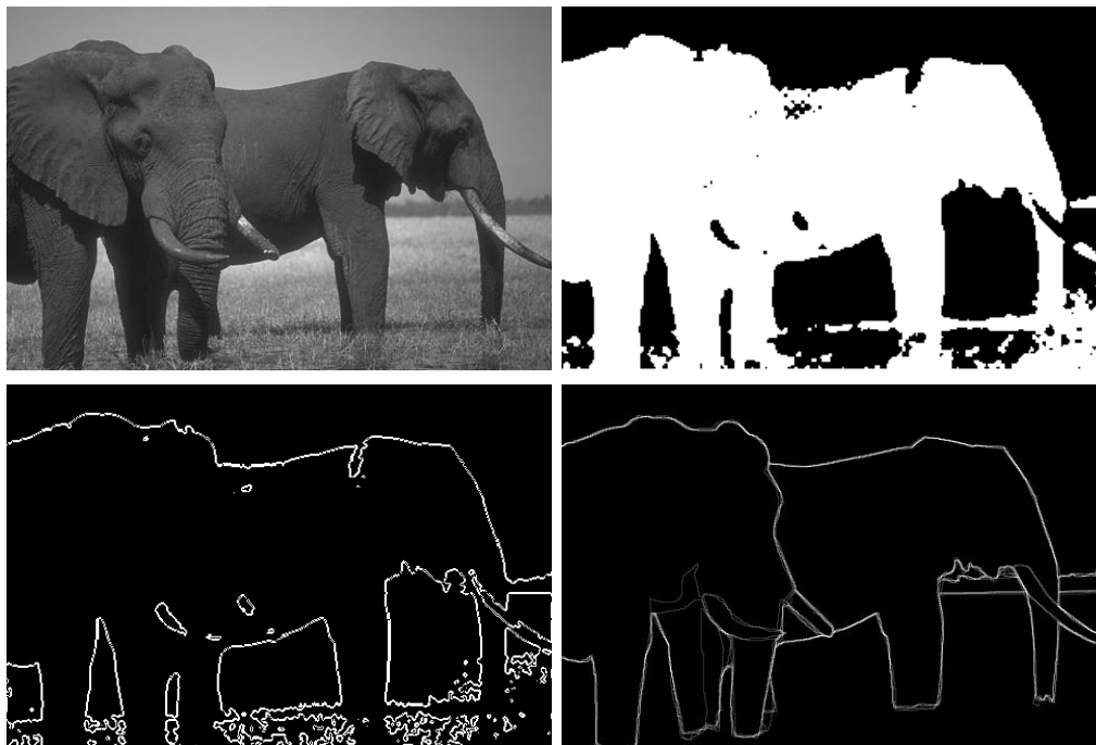
Figure 5.7: 2D image segmentation results: (1) 2D origin image (2) the Chan-Vese method (3) the proposed method (4) reference.
