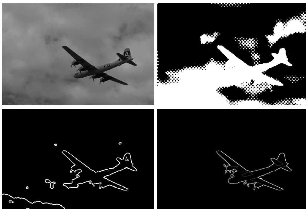
Figure 5.8: 2D image segmentation results: (1) 2D origin image (2) the Chan-Vese method (3) the proposed Method (4) reference.
