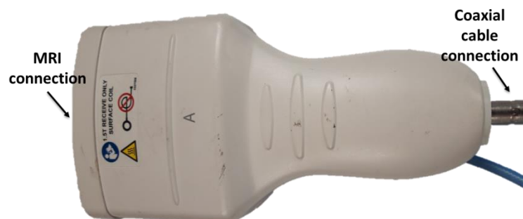
Fig. 1-9. An interface connector type of A-Plug (GE Healthcare Inc.).
