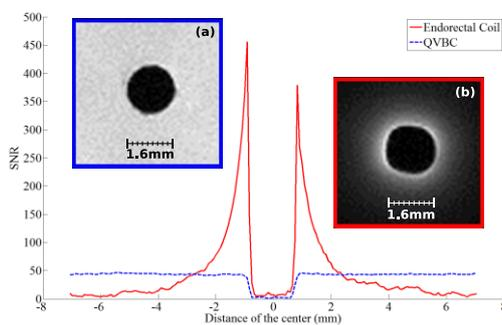
Figure 2 – SNR profiles of the EC (blue) and QVBC (red) obtain on the phantom containing only the solution.
