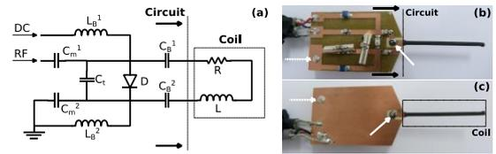
Figure 1 – Electronic scheme (a) and pictures (b and c) of the EC.
