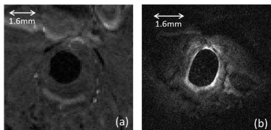
**Figure 3** - Images obtain with (a) a quadrature volume birdcage coil and (b) with the endoluminal coil, T<sub>1</sub> FLASH sequence. At the edge of the coil, the SNR is 4 times greater with the endoluminal coil.
