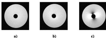
**Figure 4.** Axial images of a phantom obtained using GRE sequence with: a) A galvanic-decoupled coil. b) An optically-decoupled coil. c) A coupled coil.
