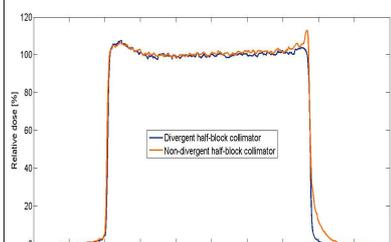
Fig.2: Comparison of dose profiles acquired in **Uniform Scanning** for divergent and non-divergent half-block collimators for a range of 20 cm in water and 4 cm air-gap.
