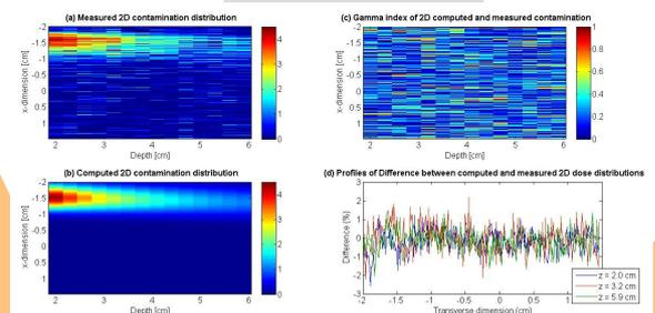
Fig.3: Comparison of the measured (a) and calculated (b) entrance face collimator contamination for a half-block collimator at range of 16.9 cm in Double Scattering. (c) 2D Gamma index computation. (d) Mean difference 1D profiles between the both distributions show 0.18% in average of difference.
