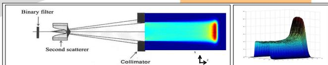
Fig.1: Measurements of 2D dose distribution for a pristine Bragg peak through a 3 cm diameter circular aperture (DS).
