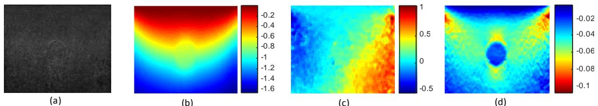
**Figure 1:** Example of results obtained on a breast mimicking phantom imaged with ultrasound imaging and subjected to slow axial compression. The scanned plane crosses a spherical inclusion that is stiffer than the surrounding material. (a) Conventional ultrasound image, (b) Axial displacement (mm), (c) Lateral displacement (mm) and (d) Axial strain, where the inclusion is clearly brought out compared to the conventional ultrasound image.
