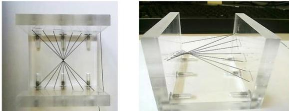
Figure 3 – Top and side view of the wires phantom consisting of 7 wires used to have data with different orientations.
