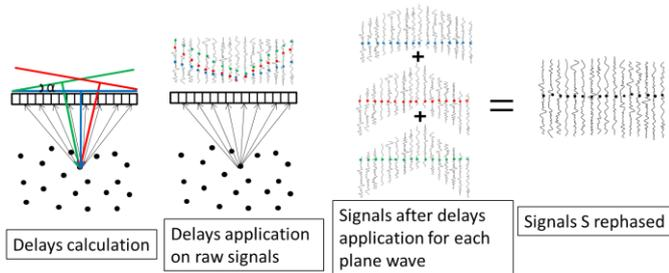
Figure 1 – Plane waves coherent compounding in order to create a synthetically focusing in emission and in reception.
