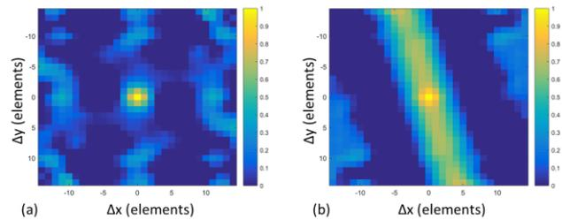
Figure 2 – Coherence function in 2D in a point of an (a) isotropic medium and (b) anisotropic medium.
