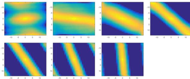
Figure 4 – Coherence functions for a point in the center of the probe corresponding to the depth of each wire of the wire phantom. Results are obtained in diverging waves.
