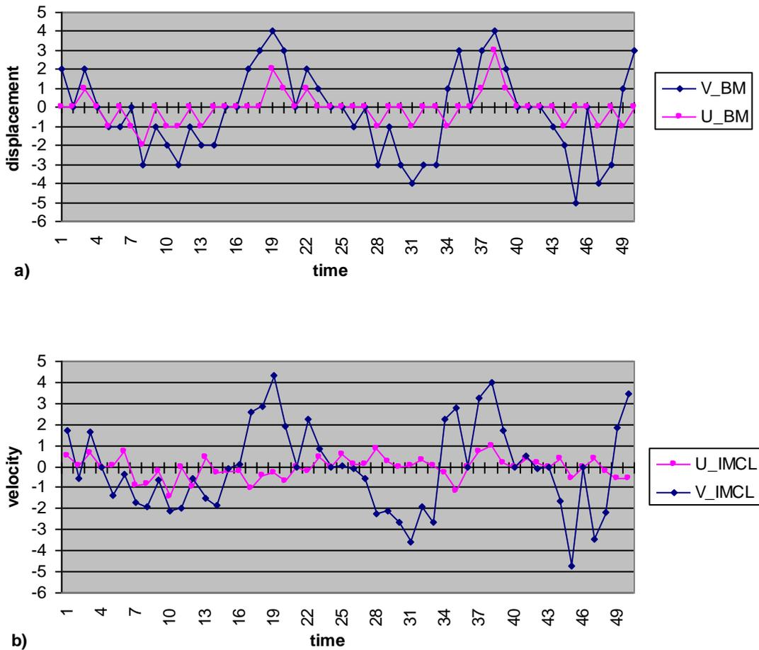
Figure 6 : Displacements (velocities) of the tumor from fig.2a, estimated by the BM algorithm (a) and by the IMCL algorithm (b). Displacements along the X-axis are negligible, while the displacements along the Y-axis show the same periodicity and magnitude in both graphs.
