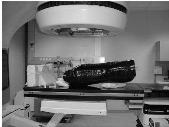
Figure 4 : Experimental setup for image acquisition of a human-body phantom. Top down : collimator of the accelerator, phantom, mobile table with position controlled by electrical drives. The imaging device is placed below the table.
