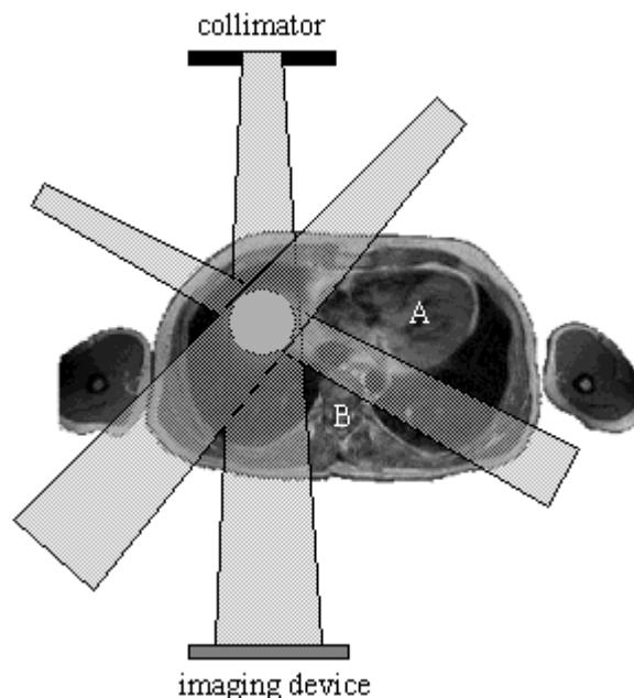
**Figure 1** : Scanner cross-section of human thorax with a schematic representation of a radiotherapy treatment setup. An electronic portal imaging device (EPID) can be placed in front of the collimator and moved around the patient, following the beam orientation changes. Planned beam orientations avoid irradiation of vital organs such as heart (A) and spine (B).
