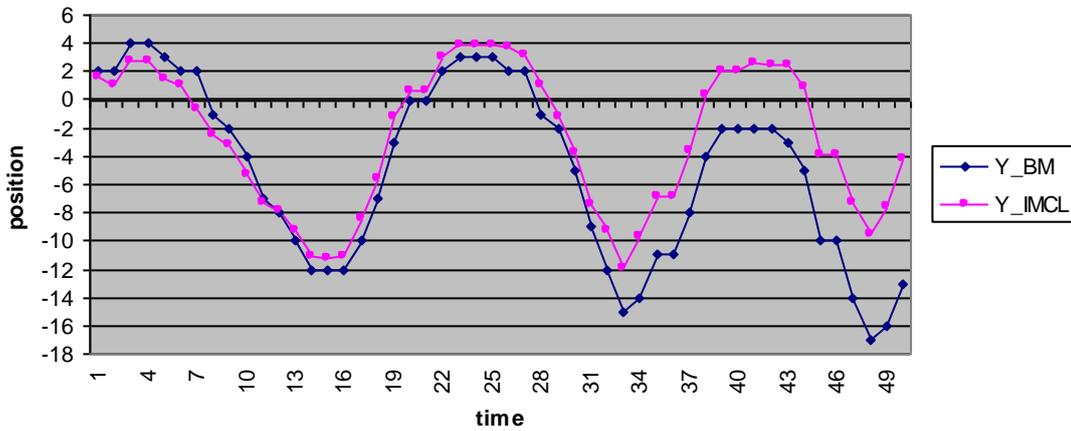
Figure 7 : Trajectories along the Y-axis obtained by integrating the velocities from fig.6.
