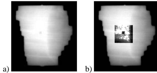
**Figure 5** : Portal image of the phantom, obtained by a conventional EPID (Varian, Palo Alto, USA). The implanted marker is hardly perceptible in the image (a). Histogram equalization of the central part of the image highlights the marker (b).
