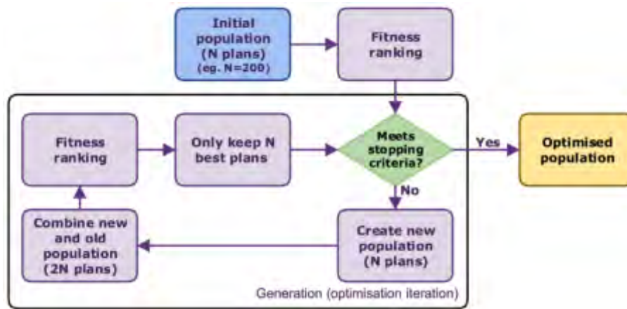
Figure 2.13: Schematic of NSGA-II. New populations are created by mixing solutions from the previous population. The new and previous populations are added together, sorted and the best half are kept, whilst the worst half are discarded.
