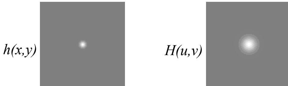
Isotropic low pass filter with poor selectivity H(u,v) is a gaussian
