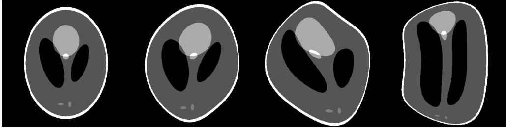
Figure 4. The deformed phantom visualized at different moments during the measurement. Due to different angular conventions here and in [11], the motion was parameterized by (\beta - \pi/2) \bmod 2\pi instead of just \beta . From left to right: \beta = 90^\circ (reference time), \beta = 210^\circ , \beta = 10^\circ , \beta = 89^\circ .
