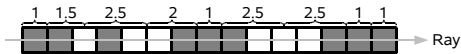
Fig. 3. Weighted sum of voxel intensities (grey) of the sheared volume along the ray when there are holes (white).
