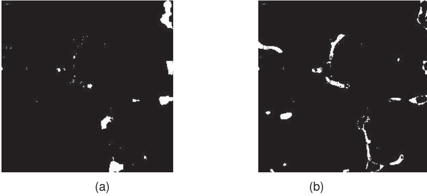
Figure 9: (a) Best reconstruction of the low density image obtained with the the nonlinear diffusion equation ( A_4 ) for \sigma_p = 20 , and M = 10 projections, MR = 2.63\% ; (b) Corresponding error map.
