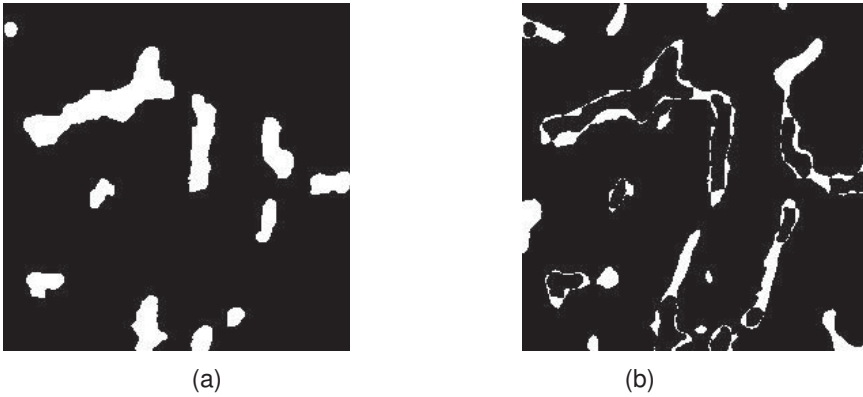
Figure 2: (a) Reconstruction of the high density image f_0 obtained with the TV regularization for \sigma_p = 20 (PPSNR=6 dB) and M=10 projections, MR = 8.12\% ; (b) Corresponding error map.
